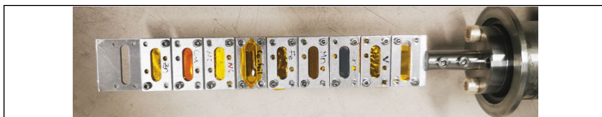
Figure 4: 3d reference metals sample holder with all the elements from Ti to Zn mounted on.
